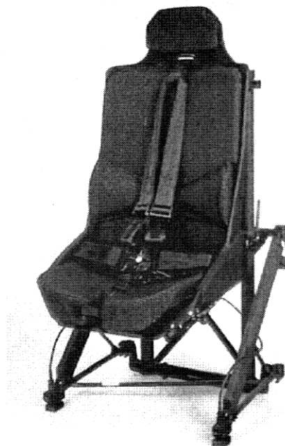
Figure 2. Crew seat from a UH-60 Black Hawk helicopter used for drop testing.
